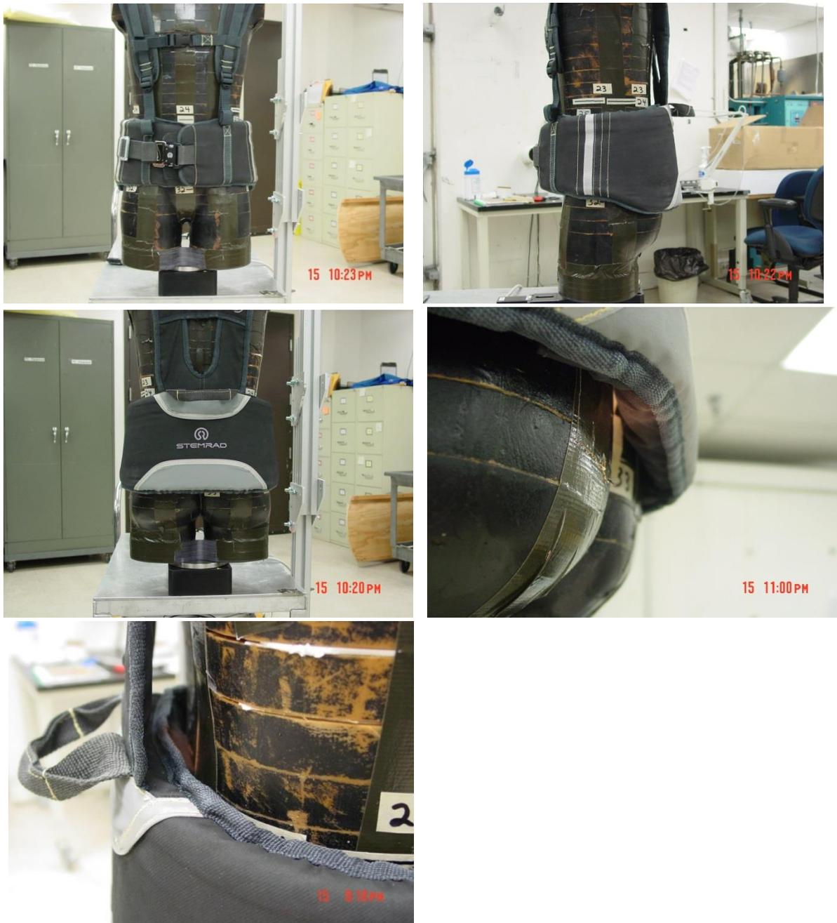
**Figure 1. Photos of small-sized belt on RANDO® phantom. These photos allowed StemRad staff to verify that the fit met with their specifications.**
