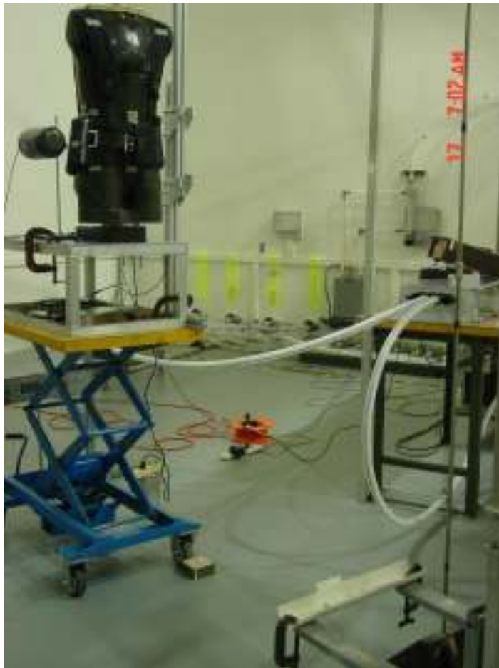
Figure 2a. Photo of wide view of actual setup just prior to irradiation Run #2, with RANDO (belt ON) on left, and white PVC source holder on bottom right.
